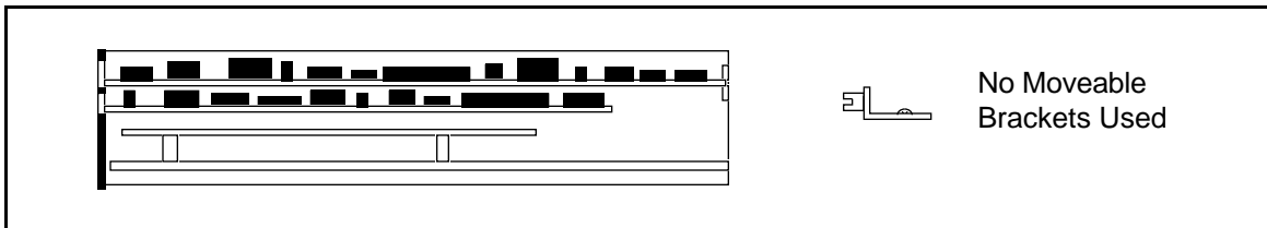
Figure F-15. First Board between 8.2 in. and 13.4 in. Long, Second Board Full 13.4 in. Long
