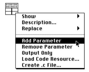
Each pair of terminals corresponds to a parameter that LabVIEW passes to the CIN. The two types of terminal pairs are input-output and output-only.
