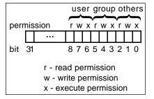
On the PC, permissions are ignored for directories. For files, only bit 7 (the UNIX user write permission bit) is used. If this bit is clear, the file is read-only. Otherwise, you can write to the file.
