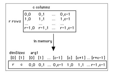
For an array with r rows and c columns, you can access the element at row i and column j as shown in the following code fragment.
