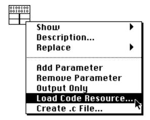
This command loads your object code into memory and links the code to the current front panel/block diagram. After you save the VI, the file containing the object code does not need to be resident on the computer running LabVIEW for the VI to execute.
