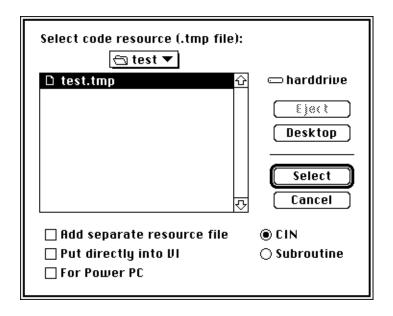
If you are making a CIN, select the **CIN** option in the dialog box, as shown in the preceding illustration. If you are making a CIN for the Power Macintosh, also check the **For Power PC** box. If you are making an external subroutine, select the **Subroutine** option.
