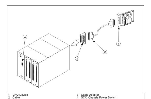
Figure 2-2. Connecting an SCXI Chassis to a DAQ Device
