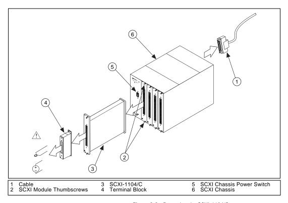
Figure 2-3. Removing the SCXI-1104/C
