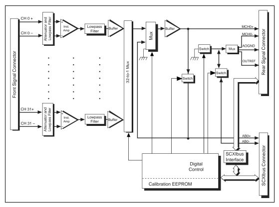
Figure 5-1. SCXI-1104/C Module Block Diagram
