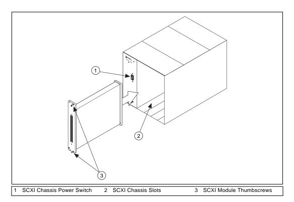
Figure 2-1. Installing the SCXI-1104/C Module
