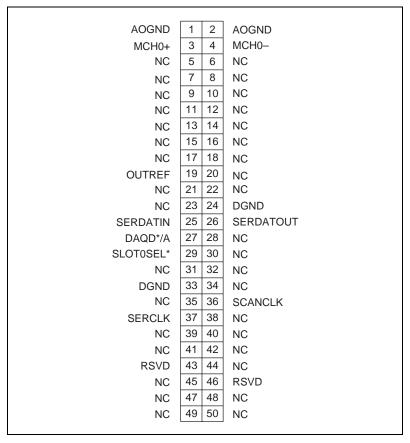
Figure 3-2. SCXI-1104/C Module Rear Signal Connector Pin Assignments
