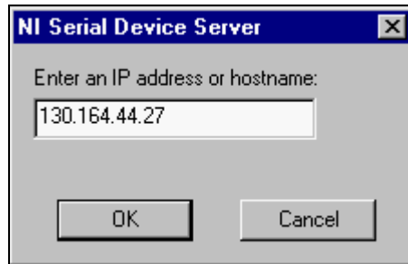
Figure 4-2. Specifying a Serial Device Server
