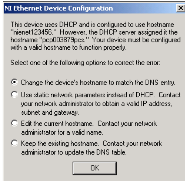
Figure 3-5. Resolving a Hostname Verification Error
