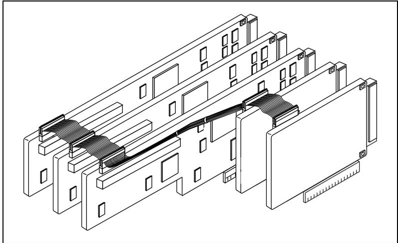
**Figure 1.** Extended Five-Board RTSI Bus Cable Setup
