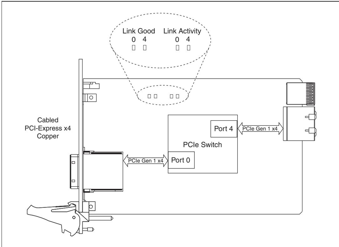
**Figure 4.** NI PXIe-8374 (193970x-02L) Onboard LED Locations
