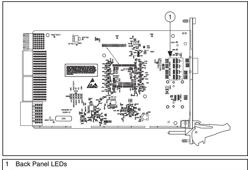
**Figure 5.** NI PXIe-8370 Back Side LED Locations
