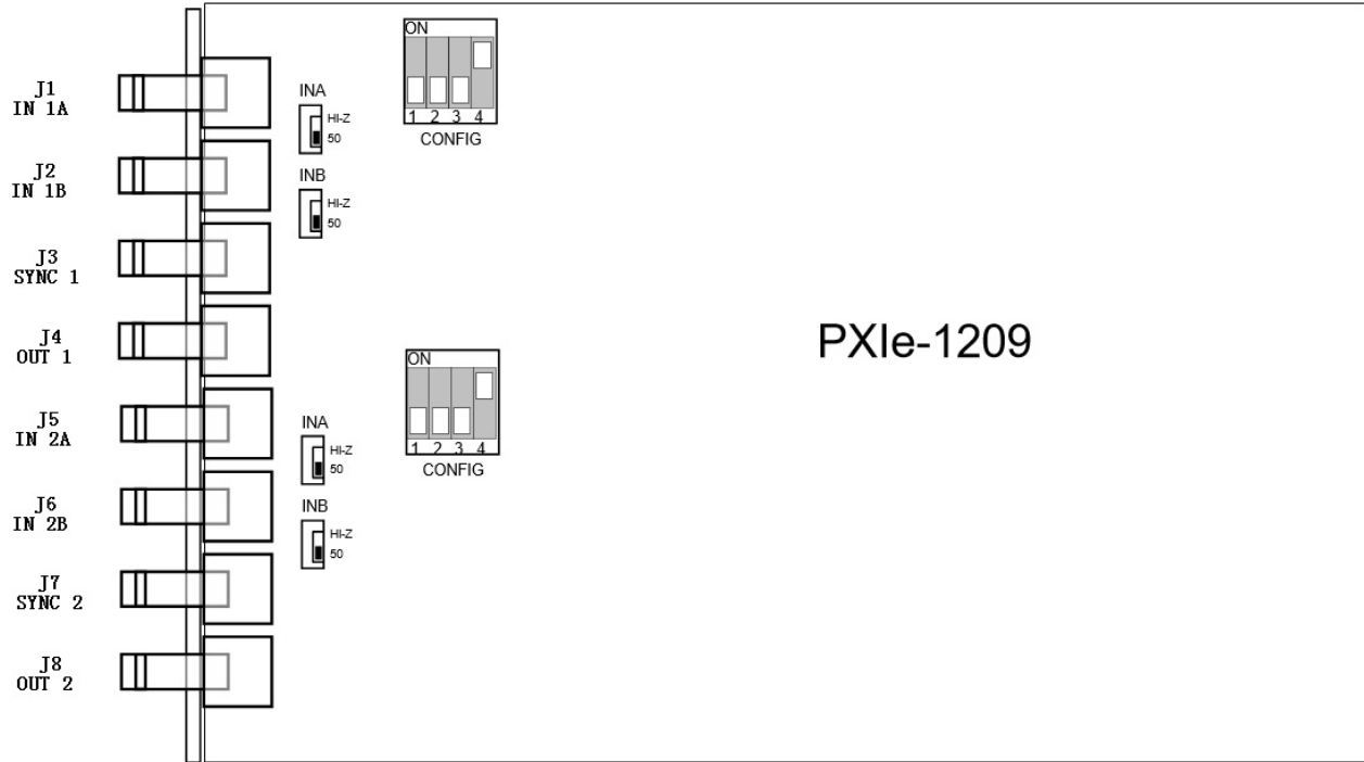
Figure 1-4, PXIe-1209 Hardware Configuration Switches
