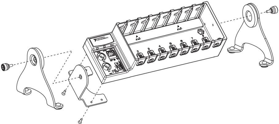
You must mount the chassis *before* installing the C Series modules.
