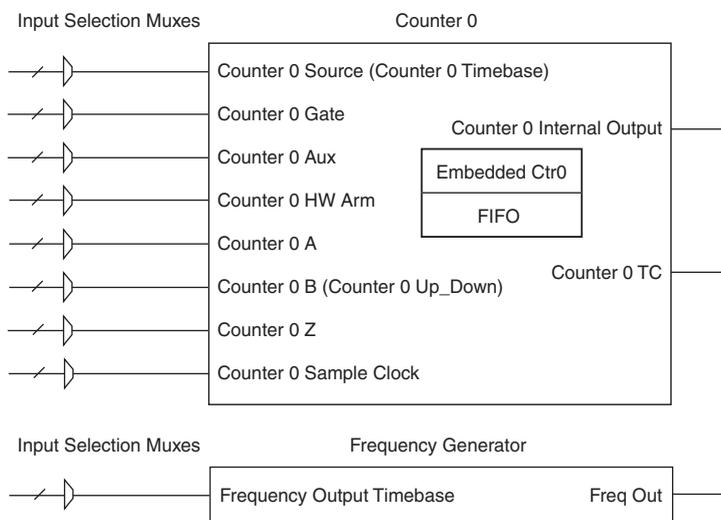
Counters have eight input signals, although in most applications only a few inputs are used.
