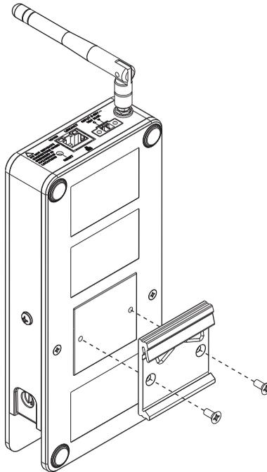
Clip the chassis onto the DIN rail with the larger lip of the DIN rail clip positioned up, as shown in Figure 1-18.
