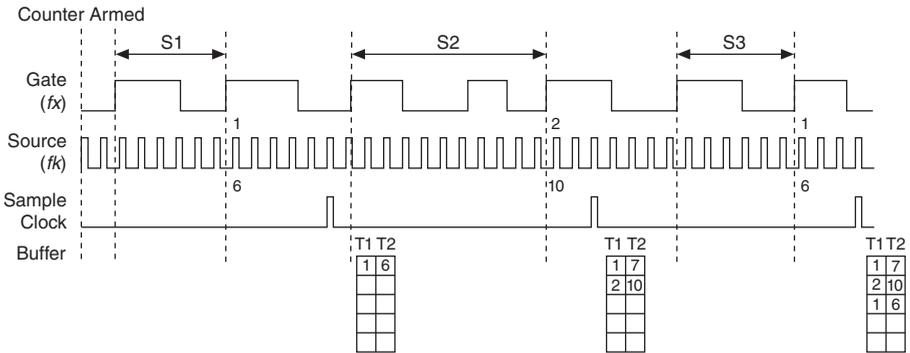
When **Cl.Freq.EnableAveraging** is set to false, the frequency measurement returns the frequency of the pulse just before the sample clock. This single measurement is a single frequency measurement and is not an average between clocks as shown in Figure 5-16.
