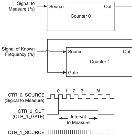
Next, route the Counter 0 Internal Output signal to the Gate input of Counter 1. You can route a signal of known frequency ( $f_k$ ) to the Counter 1 Source input. Configure Counter 1 to perform a single pulse-width measurement. Suppose the result is that the pulse width is  $J$  periods of the  $f_k$  clock.
