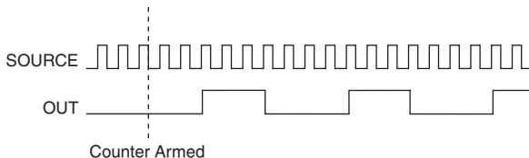
Continuous pulse train generation is sometimes called frequency division. If the high and low pulse widths of the output signal are  $M$  and  $N$  periods, then the frequency of the Counter  $n$  Internal Output signal is equal to the frequency of the Source input divided by  $M + N$ .
