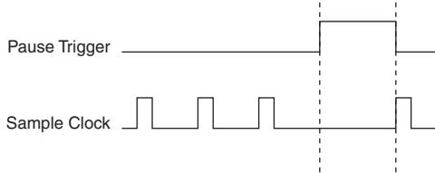
If you are using any signal other than the onboard clock as the source of the sample clock, the generation resumes as soon as the pause trigger is deasserted and another edge of the sample clock is received, as shown in Figure 3-3.
