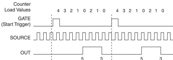
Figure 5-30 shows the same pulse train with **CO.EnableInitialDelayOnRetrigger** set to the default False.
