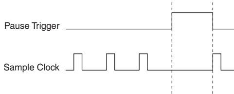
If you are using any signal other than the onboard clock as the source of the sample clock, the generation resumes as soon as the pause trigger is deasserted and another edge of the sample clock is received, as shown in Figure 4-6.
