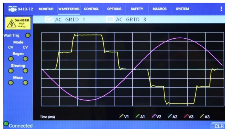
Split Phase (2- \phi ) shown with A-Phase using a n-Step sine output
