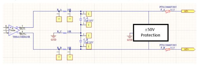
By default **C\_A** and **C\_B** are not installed, and **R\_A**, **R\_B** and **R\_C** are 10 Ohm.
