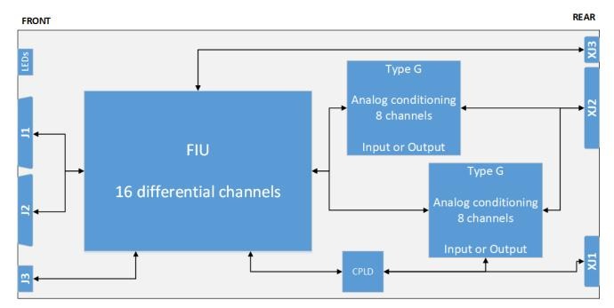
The input/output conditioning is managed by a combination of these two OP8Gxx (also called Type-G) modules:
