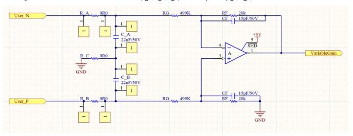
By default **R\_C**, **C\_A** and **C\_B** are not installed, and **R\_A** and **R\_B** are 0 Ohm.
