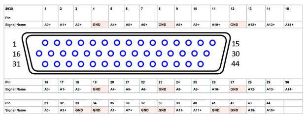
The direction of the signals A0 to A15 depend on the OP8930 assembly selected :
