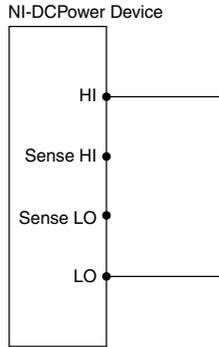
2. Set the **niDCPower Output Function** property or `NIDCPOWER_OUTPUT_FUNCTION` attribute to DC Voltage for the NI 4140.
