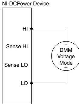
2. Set the **niDCPower Output Function** property or `NIDCPOWER_OUTPUT_FUNCTION` attribute to DC Voltage for the NI 4140.
