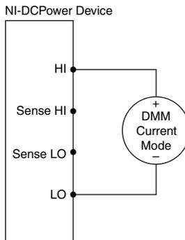
2. Set the **niDCPower Output Function** property or `NIDCPOWER_OUTPUT_FUNCTION` attribute to DC Current for the NI 4140.
