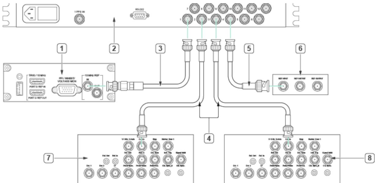
1. Timing and Sync Module of PXI Chassis
