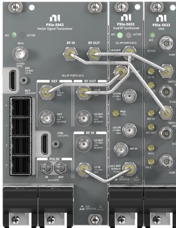
This NI VST with S-Parameters consists of a NI PXIe-5842, a NI PXIe-5655 and a NI PXIe-5633 paired as a multi-module. The calibration certificate will list the three devices.
