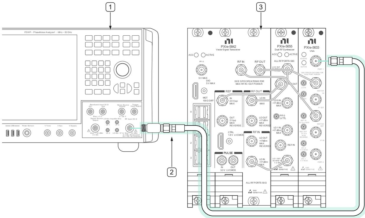
1. Phase noise and Spectrum analyzer
